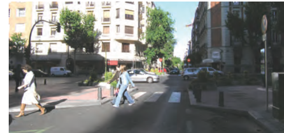
Traffic “chokers”, such as this, narrow the vehicular lane at intersections, thus forcing automobiles to slow down at pedestrian crossings.
