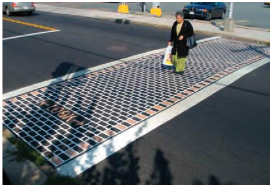
Clearly marked cross walks incorporating a change in surface material such as above and to the right not only make cross walks easier to locate, but also serve to slow down vehicles, making the crossing safer for pedestrians and calming traffic in general.
